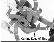
Figure 5-7: Removing tine assembly.
